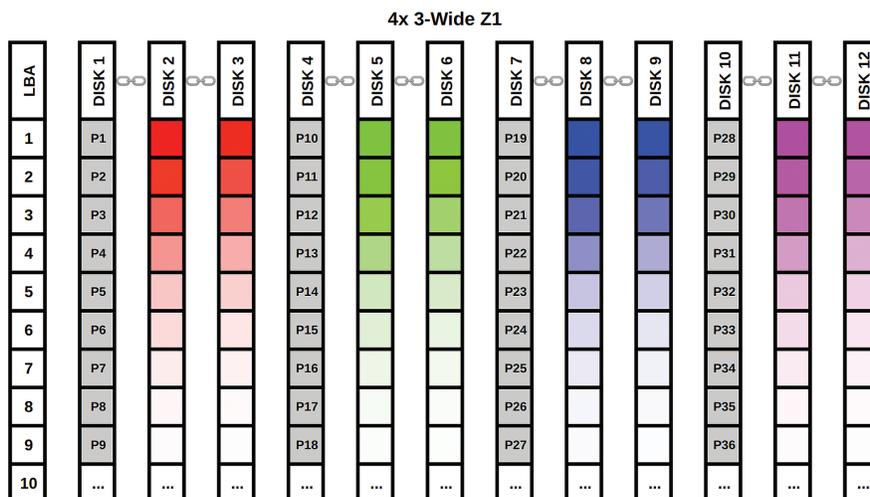
Each stripe gets its own parity sector, but unlike the previous examples, we only have a single parity sector per data stripe. This is why RAIDZ1 is not highly fault tolerant and is thus not a recommended configuration for storing mission-critical data.
