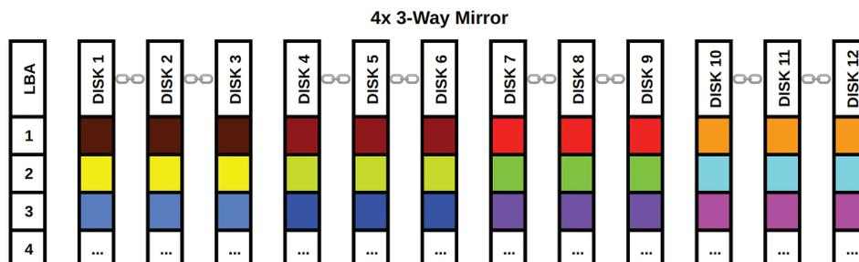
While we have sacrificed some write performance and capacity, the pool is now extremely fault tolerant. This configuration is probably not practical for most applications and it would make more sense to use lower fault tolerance and set up an offsite backup system.
