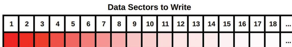
This single data block is shown as continuing on past its 18th sector with the ellipsis at the end of the block. We have represented it this way because ZFS uses variable block sizes when writing data to vdevs. This has important implications in ZFS deployments, particularly for RAIDZ configurations. For now, let's look at general RAIDZ performance. Here's a summary:
