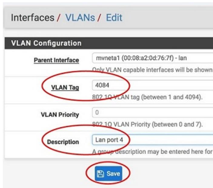
**Note:** 4084 is used as an example in this guide. The value for the tags must be unique for each VLAN and must be between 1 and 4094. Avoid using values that are already in use. Best practice is not to use 1.
