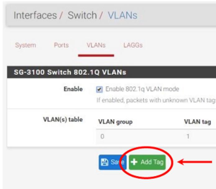
18. Type 4084 for the **VLAN Tag** and 4 for **Member(s)**. This represents LAN4 (port 4) and tagged should be **unchecked**.
