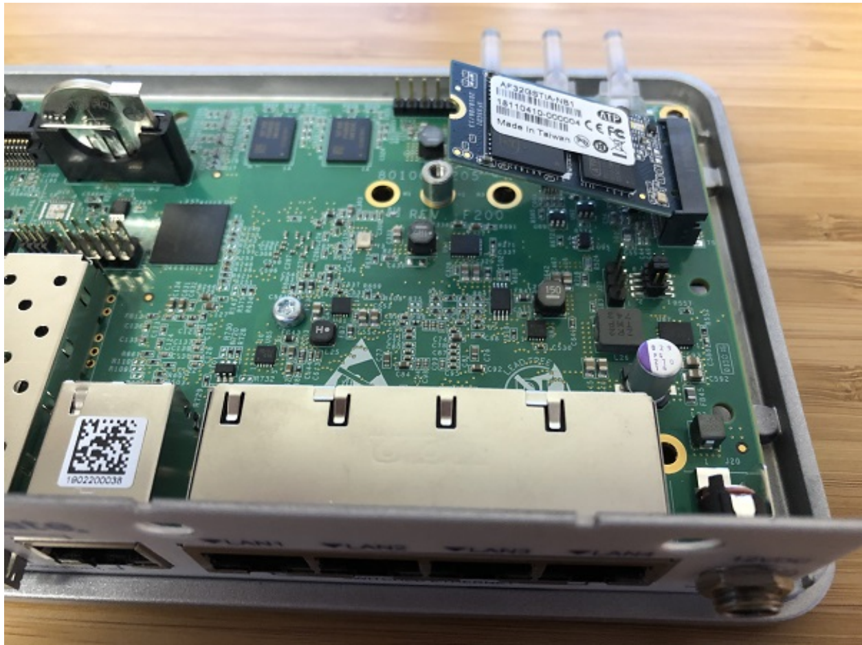
Fig. 3: Insert the M.2 SATA Drive at about a 30° Angle
