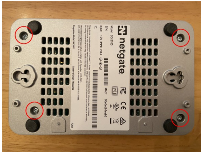
Fig. 1: Removing the SG-2100 Case Screws
